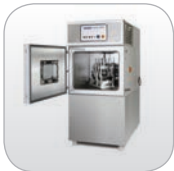
CRT-LH4PT-BB Large Hydraulic Four Point Bending Machine
